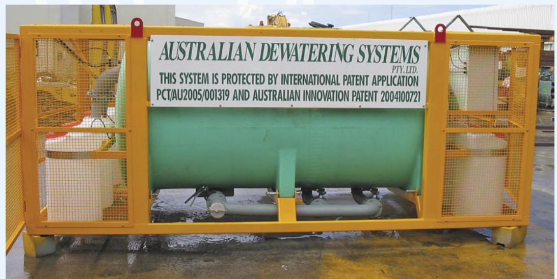
Below: ADS's patented groundwater filtration and monitoring unit.
